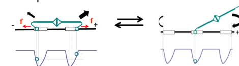
Figure 1. Design principle. (A) Three size-controlled modes of a symmetric bipedal nanomotor interacting with a periodic track of asymmetric binding sites. The motor and track are schematically illustrated in cyan and black; the underlying blue lines show the binding free energy between a motor leg (empty circle) and the binding sites (empty rectangles). A leg-site binding is asymmetric in that it is broken more easily when the leg is pulled from one end of the track than the other end. This asymmetry amounts to a binding free energy that changes more steeply along one edge than the other. As an example, the two edges are shown here as harmonic oscillator potentials with a lower elastic constant for the edge near the track's plus end as indicated. The size of a motor limits its leg-track interaction to different modes: a short motor (compared to the binding site period) explores the two inner edges of adjacent sites (contracted mode); a long motor explores the two outer edges. The same internal tension ( f ) of a two-leg bound motor causes more displacement along the less steep edge and does more work to raise the free energy, resulting in a lower barrier hence a higher rate for leg dissociation along this edge than the other one (higher rates indicated by larger size for bold, filled arrows). But the dissociated leg accesses the less steep edge more easily too, and binds the track along this edge by a higher rate. The dissociation and binding have opposite preference within either mode, yielding no net direction (detailed balance). (B) Multiple regimes for a unidirectional motor by switching it between the modes. The empty arrows indicate the operation cycles: A1 \rightarrow B1 \rightarrow C1 \rightarrow D1 \rightarrow A1 for regimes R1, A2 \rightarrow B2 \rightarrow C2 \rightarrow D2 \rightarrow A2 for R2, B1 \rightarrow C1 \rightarrow C2 \rightarrow B2 \rightarrow B1 for R3, and the reverse cycle for R4. For R1 and R2, the ending states of their cycles (A1, A2) are shown to have the motor in a different position from the starting states in order to reflect the motor's net direction. The leg binding forming the ending state ( D1 \rightarrow A1 , D2 \rightarrow A2 ) can occur either forward or backward by equal chance; the motor's net direction comes from the bias in the leg dissociation ( B1 \rightarrow C1 , B2 \rightarrow C2 ).
